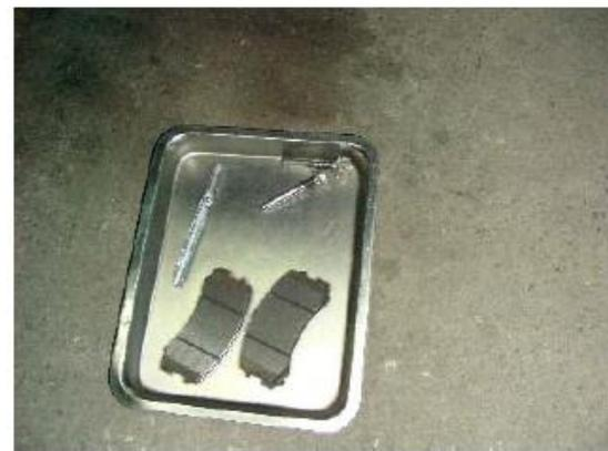
3 拆下煞車塊
